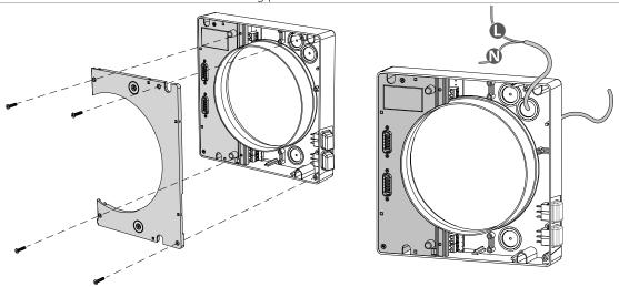
4. Using the cardboard template supplied, mark the holes for attaching the ventilator as shown in the figure below. Drill the holes and insert the dowels. Install the mounting plate unit on the wall, while laying a sealing gasket under it, fix the unit with self-tapping screws from the mounting kit. Install the mounting plate back with the connectors in place and secure it with four screws.
