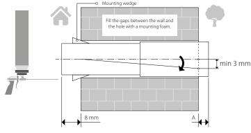
Insert the air duct into the wall as shown in the picture on the left. Install the air duct with the minimum slope of 3 mm down towards the street.
