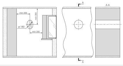
2. Insert the air duct in the wall. For ease of installation use the mounting wedges included in the delivery set. The air duct end must protrude for the distance A that enables installation of an outer ventilation hood. The distance A is stated in the installation instruction for the ventilation hood.
