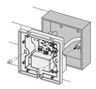
5. Fix the sensor board on the casing, and then the glass panel by pressing it until it is fixed with the latches.
