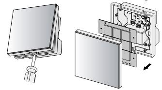
4. Attach the control panel frame to the mounting box with the screws. The fastening screws for fixation of the control panel to the mounting box are included in the delivery set.
