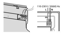
**Wall surface mounting:** lay required wires and cables to the installation place, bore the holes and fix the mounting box on the wall using the screws (separate order).
