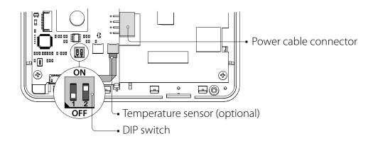
The temperature sensor is an optional device which measures the temperature in the room. If physically present in the panel configuration, select "Sensors in control panel" item in the control panel menu.
