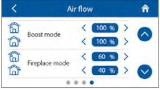
This menu enables setting the air flow rate for pre-set speed 1, 2, 3.. as well as the **Standby**, **Boost**, and **Fireplace** modes.
