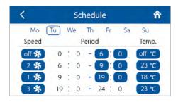
The weekly schedule contains four time periods for each day of the week. Once the weekly schedule is enabled in the Main page window, the air handling unit will run to a schedule using the following parameters:
