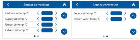
The sensor readings are corrected by entering values with horizontal arrow keys in the range from -50.0 °C to +50.0 °C.
